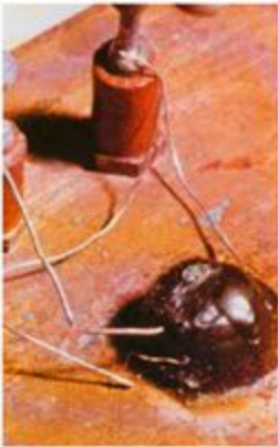
The first junction transistor (Bell Labs, 1950)
