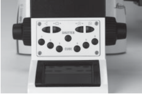
Fig. 3a Front control panel
