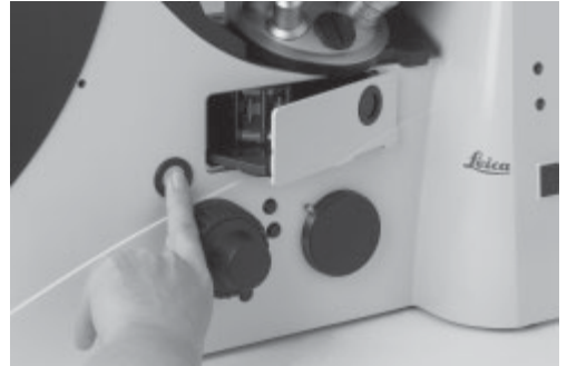
Fig. 68 Inserting or removing a filter cube
